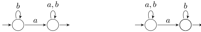
■ Figure 1 The language A^*aA^* can be recognized by a deterministic (left) or codeterministic (right) automaton, but not by a reversible one.
